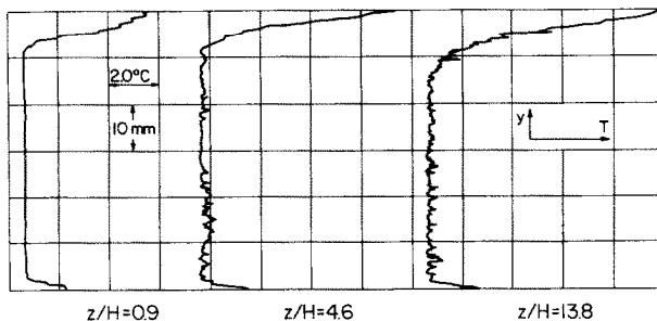
FIG. 2. Vertical temperature distributions for q_b = q_t = 1000 \text{ W/m}^2 , w_m = 10 \text{ mm/s} , H = 60 \text{ mm} , Re_H = 650 and Gr_{H,q} = 7.0 \times 10^7 .
